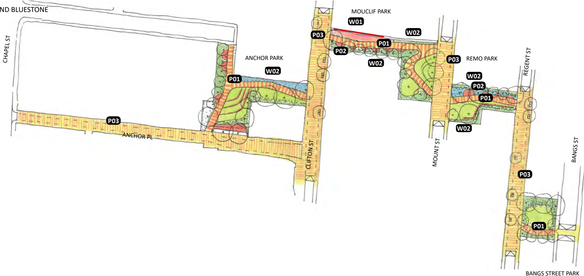
P03 - SHARED STREET PAVING NATURAL STONE 'SETT' PAVING IN TWO COLOURS, DARK GREY BLUESTONE AND SILVER GREY GRANITE SIZE: 100x100x90mm ARRANGED IN BOLD STRIPE PATTERN GRADE: VEHICLE SOURCE: LOCAL BLUESTONE AND GRANITE
