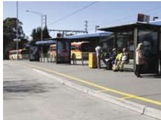
Figure 40: Parallel bus bays
