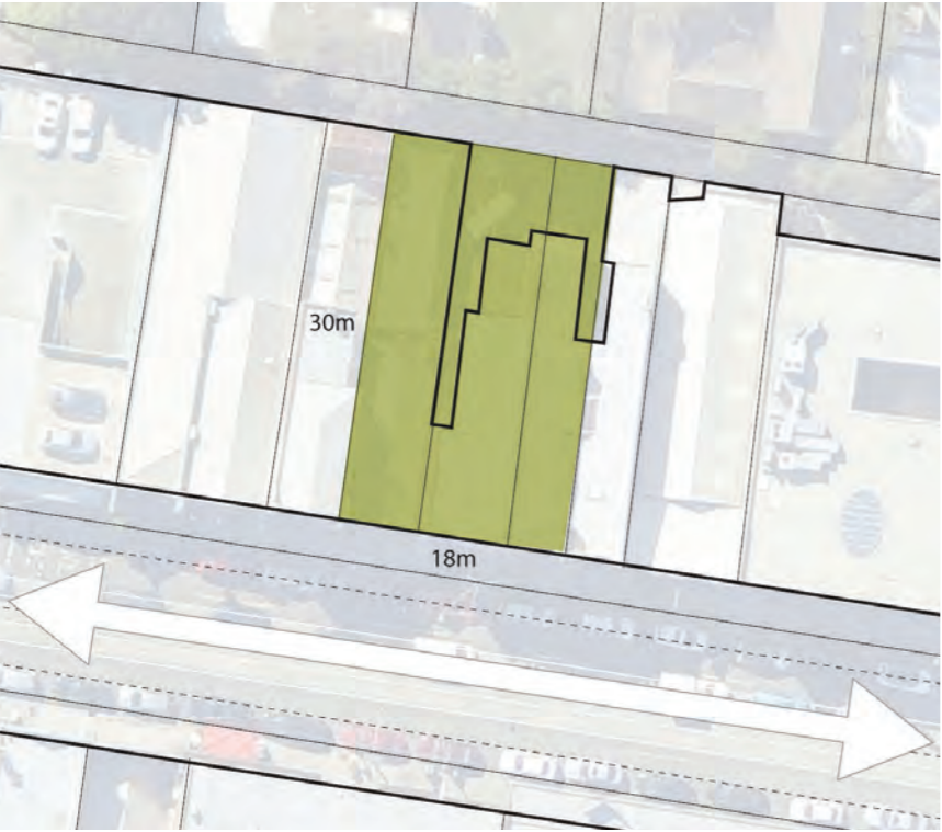
minimum typical site dimensions for a MEDIUM to LARGE allotment on High Street
