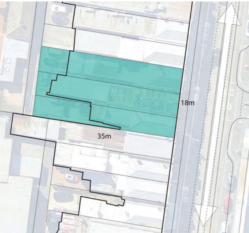
minimum typical site dimensions for a MEDIUM to LARGE allotment on Glenferrie Road
